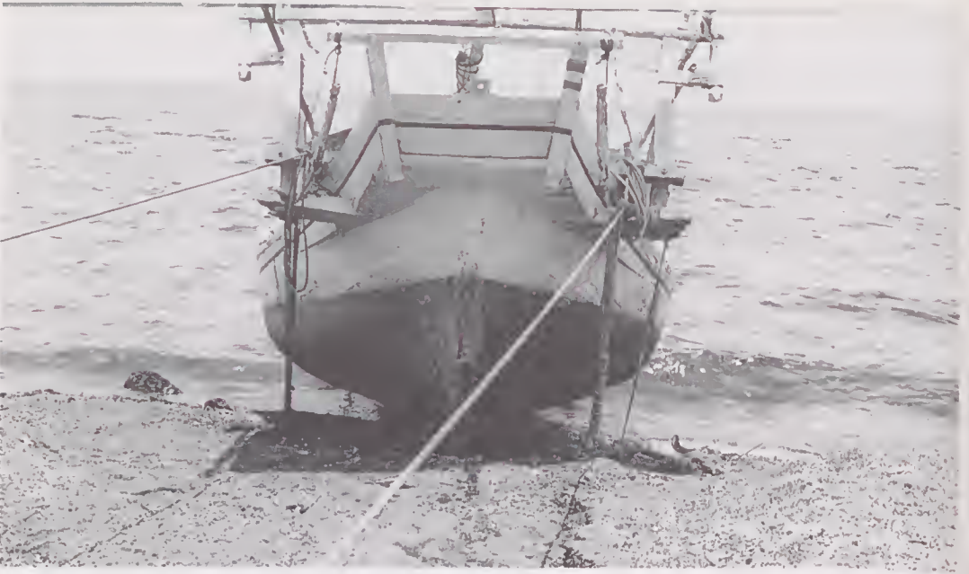
Fig. 12. The stern of a large sopé showing a typical midsection.
